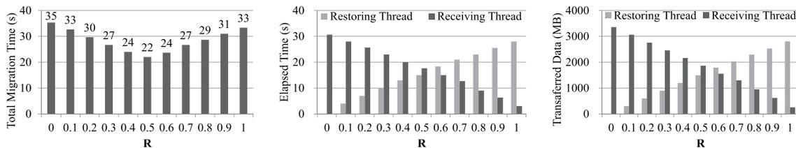
**Fig. 6** Total migartion time, elapsed time and transferred data by the two communication threads in **WebServer** Workload.
