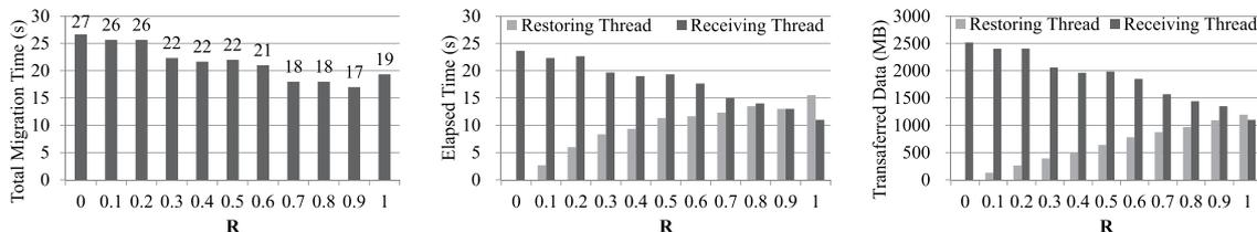
**Fig. 7** Total migartion time, elapsed time and transferred data by the two communication threads in **Postmark** Workload.
