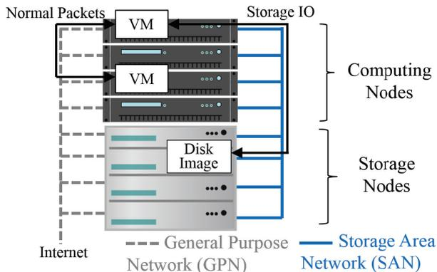
**Fig. 2** Network architecture of a data center. Storage nodes and computing nodes have designated networks: SAN and GPN.
