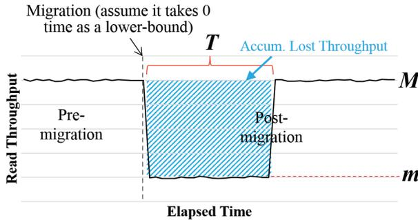
**Fig. 10** Lower bound estimation of accumulated lost throughput of a file inside a VM with existing mechanisms (dropping page cache before a migration). The read throughput degrades from  $M$  to  $m$  for  $T$  seconds after a migration, due to the loss of whole page cache. We assume the migration takes zero time, as no real implementation is available and this assumption does not break lower-bound-ness of the estimation.
