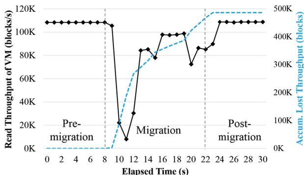
**Fig. 9** Read throughput and accumulated lost throughput of a file inside a VM before, during, and after a migration with our machanism. The throughput recovers to the max in 2 seconds after the migration. The accumulated lost throughput due to the migration overhead is 490 K blocks.
