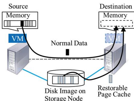
**Fig. 3** How Live Migration is Accelerated by Our Proposal. The SAN and the GPN can be used in parallel because restorable page cache can be transferred via both links.
