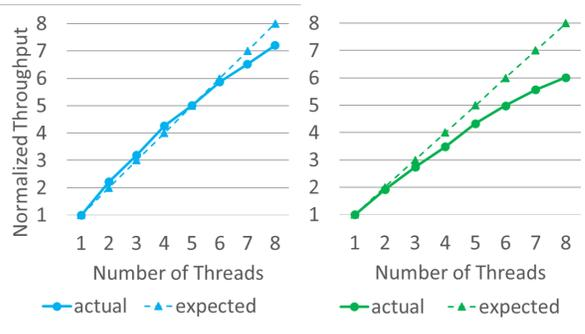
Fig. 4. Normalized Throughput of Matrix-Vector Multiplication on Machine 1 (Left) and Machine 2 (Right)
