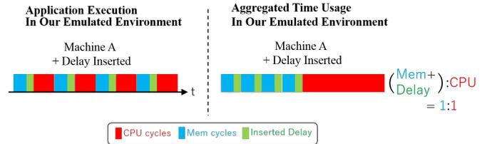
Fig. 3. The Main Idea: Delay Insertion
