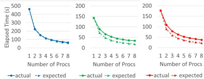
Fig. 1. Actual and Expected Execution Time of Matrix Factorization on Different Machines (two lines are overlapped in the left-most figure)
