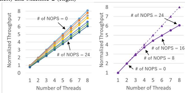
Fig. 5. Normalized Throughput of Matrix-Vector Multiplication in the Emulated Environment. Left: Each line corresponds to the number of NOPs from 0 to 24 incremented by 4. Right: Each point from  $x = 2$  to  $x = 8$  corresponds to the number of NOPs from 0 to 24 incremented by 4 (# NOPs = 0 at  $x = 2$ , # NOPs = 4 at  $x = 3$ , ..., # of NOPs = 24 at  $x = 8$ ).
